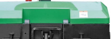
The components and connectors of the electrical system are mostly designed with high protection levels and placed inside the covering parts. The waterproof level reaches IPX4, which can meet the needs of outdoor operations.
